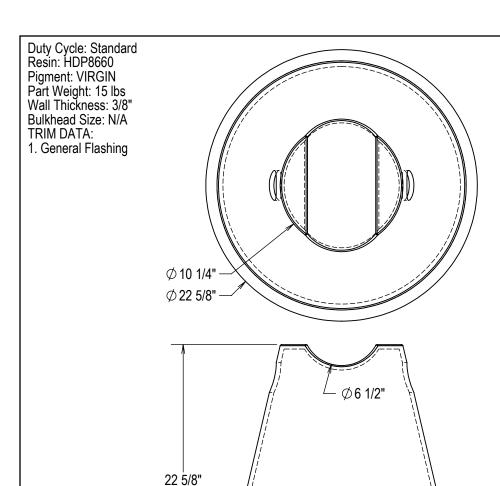
ITEM NO.DESCRIPTIONQTY.1522Resin Polyethylene HD Bulk - Tank Resin15 lbs.2814PGMNT SQUASHYELLOW,PC-4202-D3.75 G
